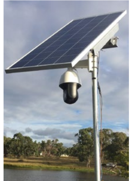
A pan-tilt-zoom security camera scans the dam for target species.
